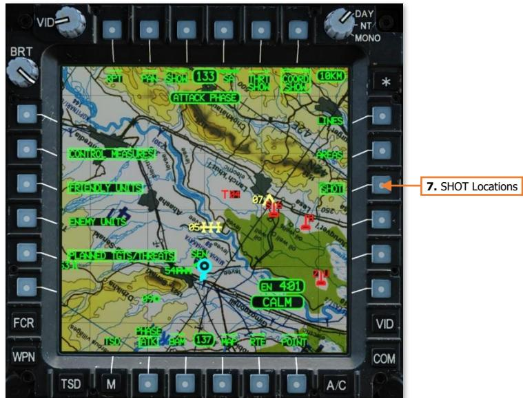
7. **SHOT Locations.** Enables/disables the display of missile engagement locations as green X symbols. Ownship missile engagement locations are displayed in full-intensity green. Missile engagement locations received via the datalink are displayed in partial-intensity green.
