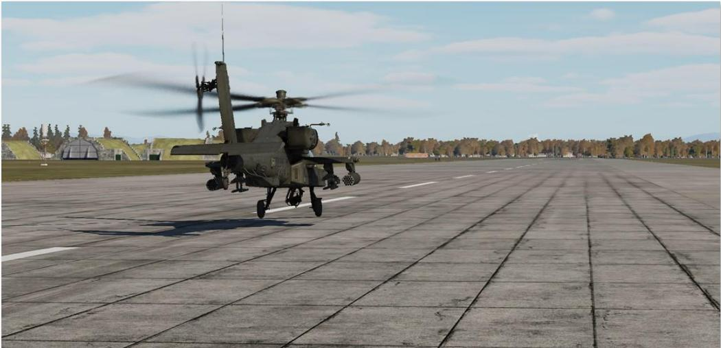
**VMC Takeoff.** A VMC Takeoff is the most common type of takeoff and can be initiated from the ground or when already established in a stationary hover. This type of takeoff is used when a sufficient power margin ( $\geq 10\%$  TQ) is available between the torque required to hover in ground effect (HOVER Q – REQUIRED IGE) and the maximum dual-engine torque available (MAX Q – DE) that does not exceed the dual-engine transmission limit (100% TQ).
