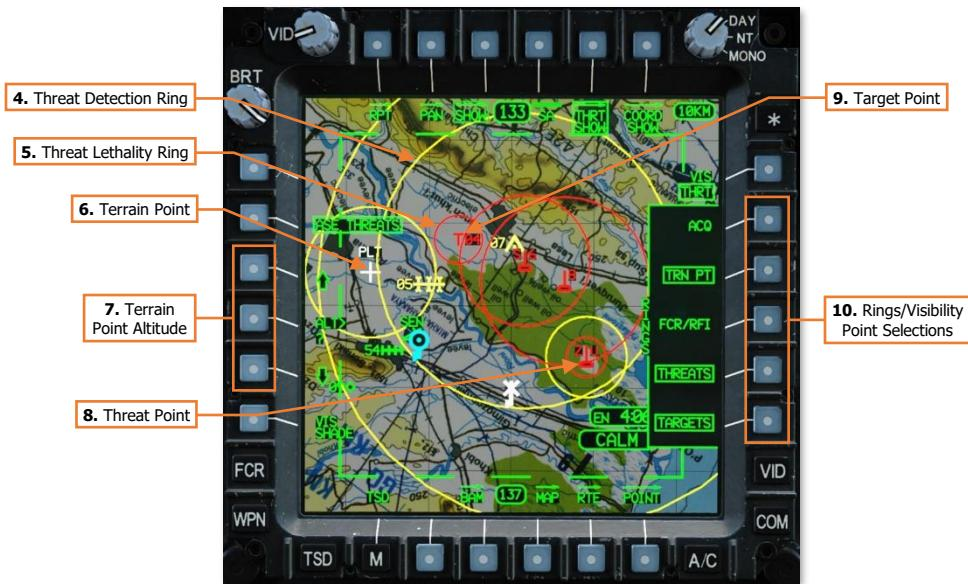
4. **Threat Detection Ring.** Yellow rings indicate the estimated range at which hostile threats are able to detect the aircraft. If VIS SHADE (VAB L6) is enabled, yellow visibility shading is drawn within the ring to display areas in which the Ownship will be visible to, and likely detected by, hostile threats based on the current aircraft altitude.
