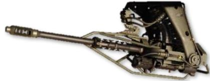
The M230 fires 30x113mm link-less, tracer-less ammunition at a rate of up to 625 rounds per minute. Ammunition is stored in a magazine in the main fuselage under the transmission and can hold up to 1200 rounds. When the Internal Auxiliary Fuel System (IAFS) is installed, magazine size is reduced to 300 rounds.
