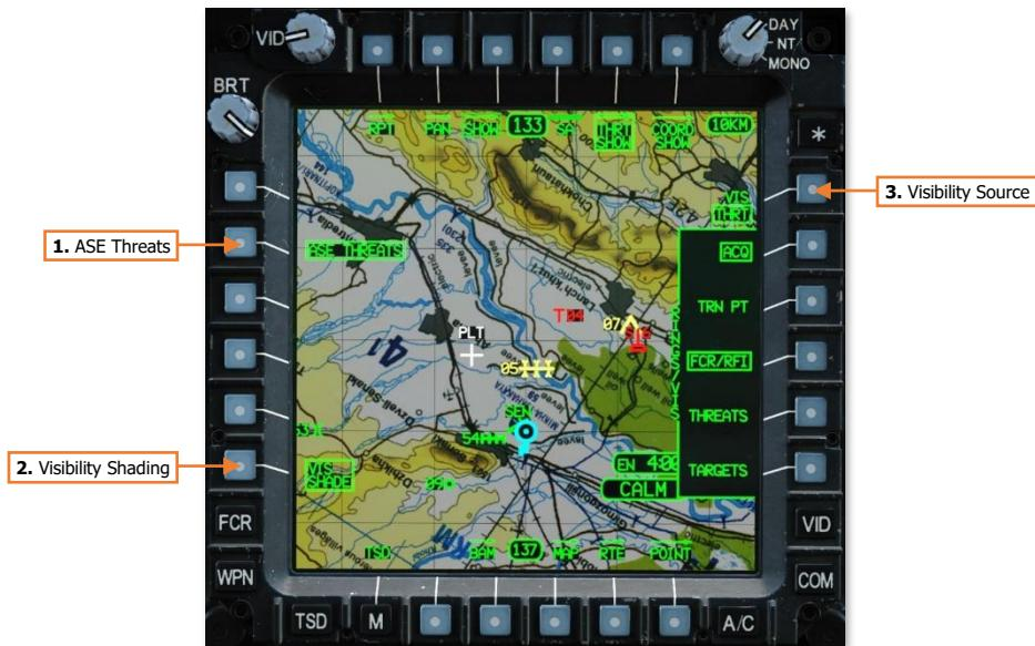
1. **ASE Threats.** Enables/disables the display of the ASE "footprint" around the outer edge of the TSD. When enabled, the ASE footprint will be displayed on the TSD if any threats are detected by the ASE system. When disabled, the ASE will still provide voice message alerts of detected threats, but the ASE footprint will not be displayed on the TSD.
