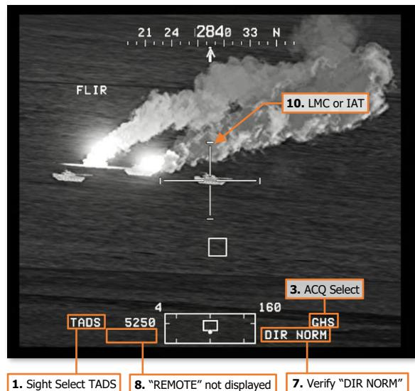
10. **CPG** If the target or aircraft are moving, engage TADS targeting modes to stabilize the TADS on target.
