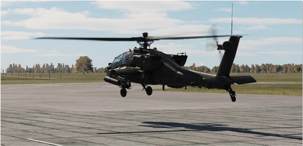
It is important to understand that when raising the collective, the torque effect from the counter-clockwise rotation of the main rotor will cause the fuselage to spin to the right. This is countered by applying left pedal, which subsequently results in the aircraft drifting to the right from the combined forces of the main rotor torque and the tail rotor thrust. This in turn is countered by applying left cyclic to hover with a slight left bank.
