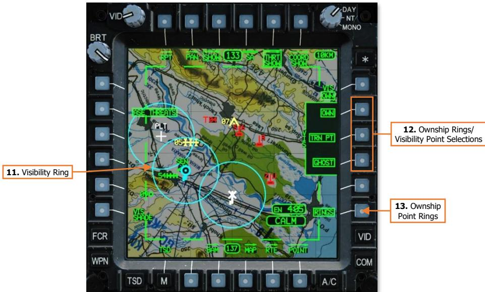
11. **Visibility Ring.** Cyan rings are displayed around the Ownship, Terrain Points, and Ghostship, if enabled by the corresponding point selections (VAB R2, R3 and R4 respectively) and the RINGS option (VAB R6).
