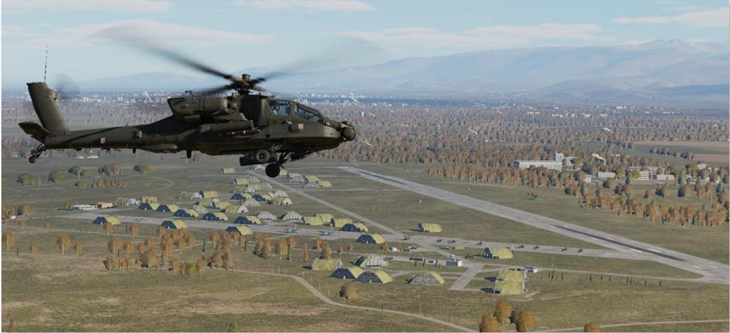
**VMC Approach.** A VMC Approach is normally performed when sufficient power margins allow for normal approach angles and deceleration prior to arriving over the intended point of touchdown. Variations in the execution of the VMC Approach are based on the nature of the landing area, obstacles around the landing area, and the whether the aircraft has the power margins to hover out of ground effect (OGE).
