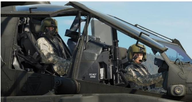
The AH-64D uses a tandem cockpit layout, with the Pilot (PLT) in the aft cockpit and the Copilot/Gunner (CPG) in the forward cockpit. Identical flight controls are present in both cockpits, and each can employ any of the AH-64's weapon systems, but the Pilot lacks several targeting and weapon employment controls that are only present in the CPG cockpit.
