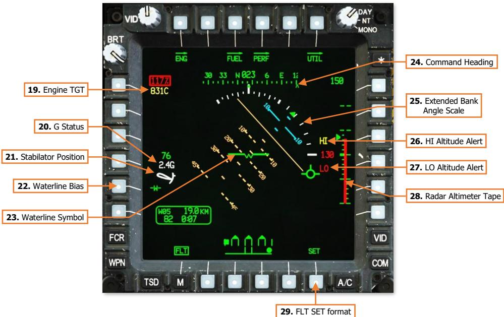
**19. Engine TGT.** Displays the highest of the two engines' Turbine Gas Temperature (TGT) indications if operating in an intermediate or contingency TGT limit.
