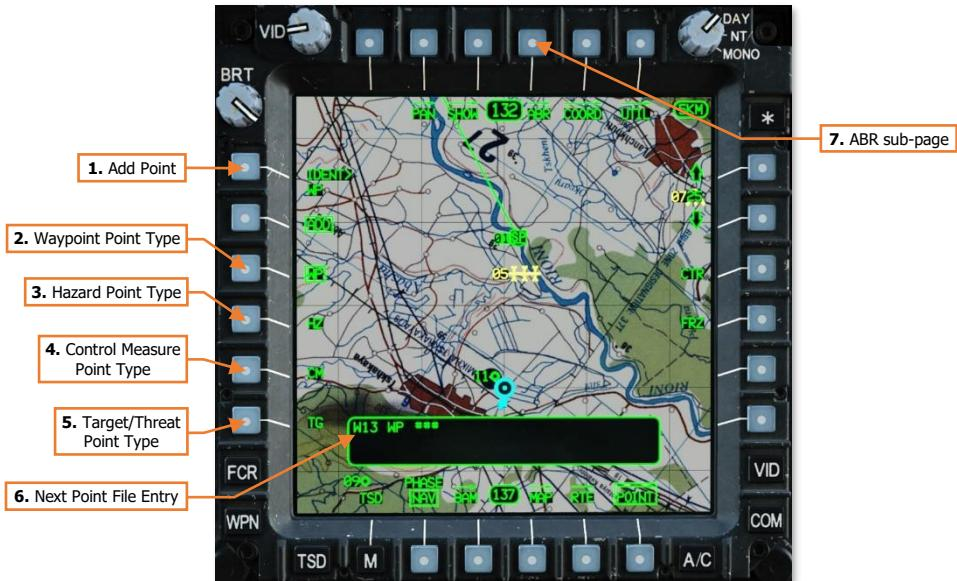
1. **Add Point.** Activates the KU for inputting new point file data. The first data element that may be input is the identifier. (See [Adding a Point using the Keyboard Unit](#) for more information.)
