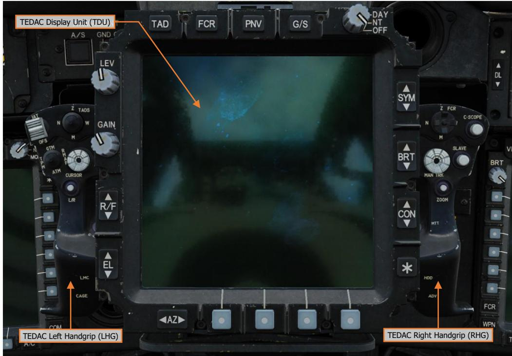
Along with the TDU bezel controls, fixed handgrips on either side of the TEDAC are used to control aircraft sensors, weapons, and the CPG's MPD cursor. Many of these controls replicate functions on the CPG's cyclic and collective controls but allow the CPG to utilize such functions without actively interfering with the Pilot's flight control inputs.
