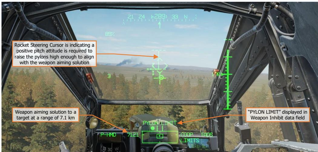
Rocket Steering Cursor is indicating a positive pitch attitude is required to raise the pylons high enough to align with the weapon aiming solution
