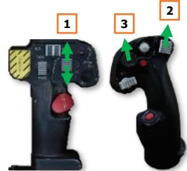
**NOTE:** When training this maneuver, increase the collective to 10% below the torque required to hover in ground effect (HOVER Q – REQUIRED IGE) to simulate a limited-power condition.
