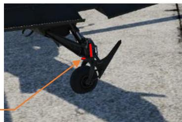
Tail wheel locking actuator cannot physically lock until aligned with tail wheel
