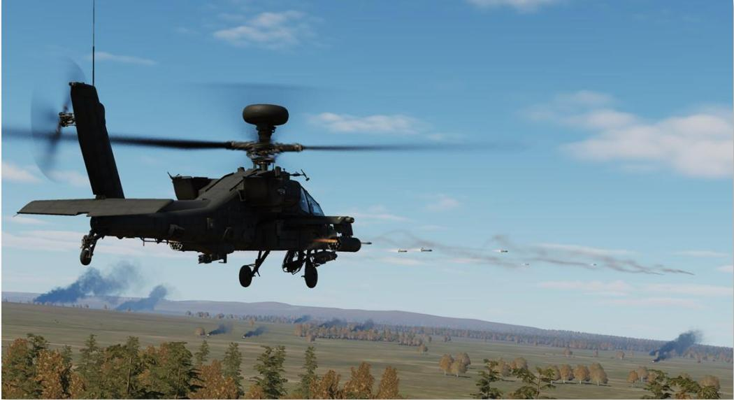
The ARS consists of up to four M261 rocket launchers (also called "rocket pods"), which are capable of firing 2.75-inch unguided rockets of the Hydra-70 rocket family. Each 19-tube pod is "zoned", which permits the carriage of up to three different warhead types when a single pair of launchers are used, or up to five different warhead types when two pairs of launchers are used. Single rocket pods may also be loaded if desired, in the case of reducing overall gross weight as necessary.
