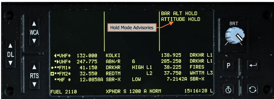
Any time the Attitude Hold or Altitude Hold are disabled using the Force Trim/Hold Mode switch, the hold mode indicators within the HMD symbology and on the FLT page will flash and an audio tone will alert the crew that a hold mode has been deactivated.
