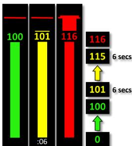
**Dual Engine Torque Limits ( $N_R > 90\%$ )**
