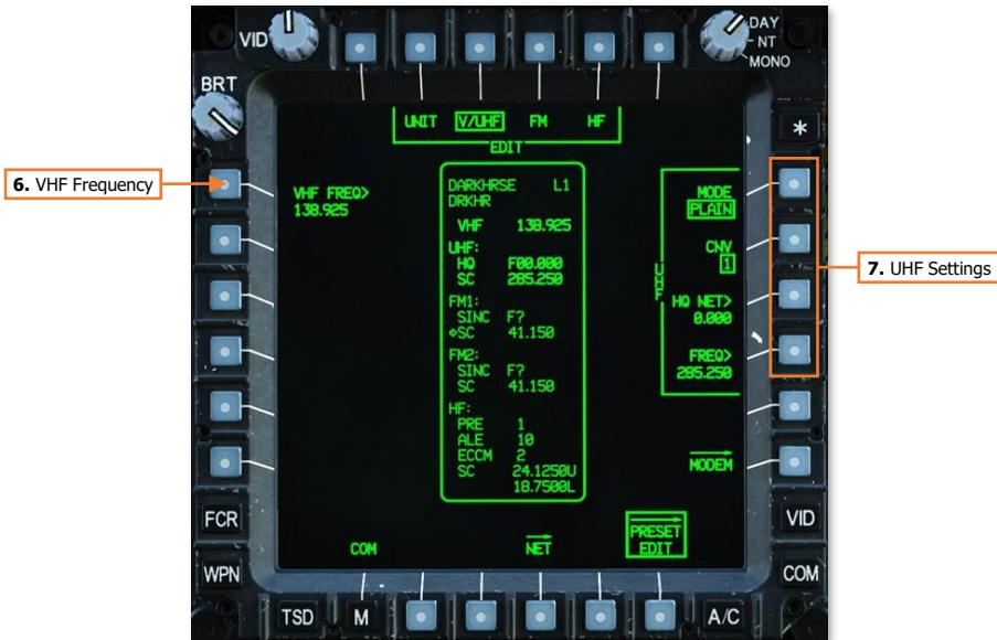
6. **VHF Frequency.** Activates the KU for inputting a VHF-AM frequency for the preset. Valid frequency entries are between 108.000 and 151.975 MHz in 0.025 MHz increments. Frequencies between 108.000 and 115.975 MHz are limited to receive-only
