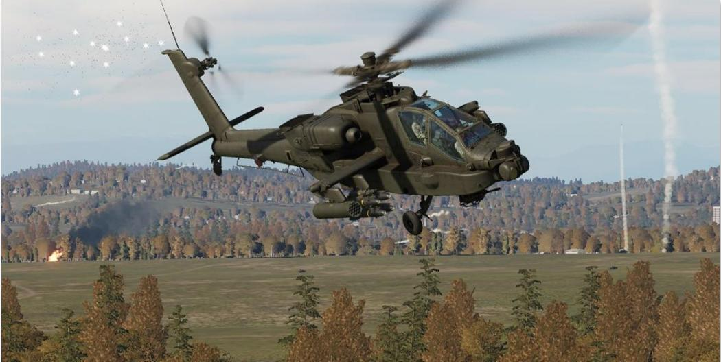
The ASE kit installed on the AH-64D includes a combined radar and laser warning receiver (RLWR), an electronic radar jamming system (ECM), a missile warning system (CMWS), chaff and flare countermeasures dispensers, infrared suppression integrated into the engine exhausts, and a Wire Strike Protection System (WSPS) installed on the forward fuselage and underside.
