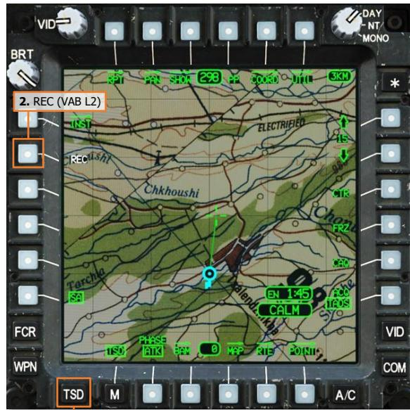
The Receive list will display the four most recent datalink messages that have not already been stored (excluding text messages and mission files). Each entry will include the type of data that has been sent within the message, the originator callsign that sent the message, and the modem protocol through which it was received.
