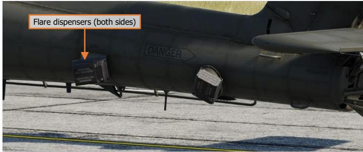
The flare dispensers utilize a pre-set flare program, which can only be modified by an external panel by ground support crews when the engines are off. Flares are dispensed using this program regardless of whether the dispensing is commanded automatically by the CMWS or manually by the aircrew.
