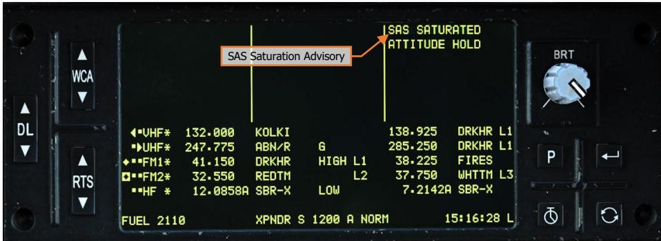
The Flight Control audio tone will sound with an associated EUFD advisory when the criteria listed below is met for each respective sub-mode:
