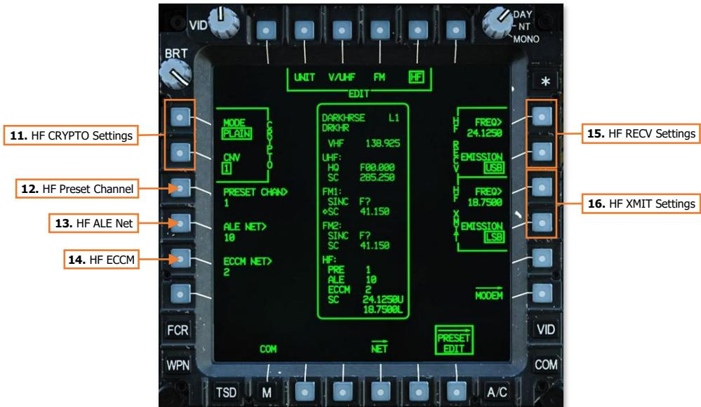
**11. HF CRYPTO Settings.** Displays settings for configuring the HF radio for secure radio communications.
