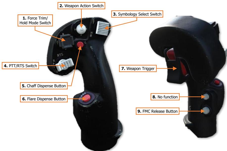
**1. Force Trim/Hold Mode Switch.** Controls the force trim and Hold modes provided by the Flight Management Computer (FMC).
