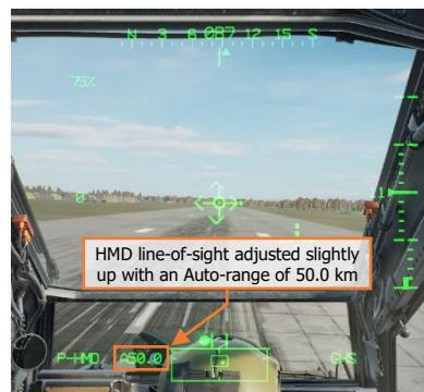
Automatic range relies upon a functioning radar altimeter and will only be usable when the aircraft's altitude above ground level (AGL) is less than 1,428 feet (the maximum altitude that is capable of being measured by the radar altimeter).
