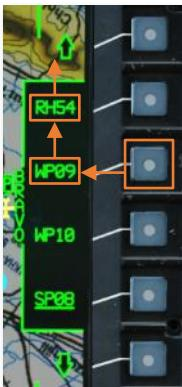
**NOTE:** When a point is inserted into a position within the route sequence that is not the END, the point that is located at that position within the route sequence will move to the subsequent position above it. All other points that follow will move to subsequent positions accordingly.
