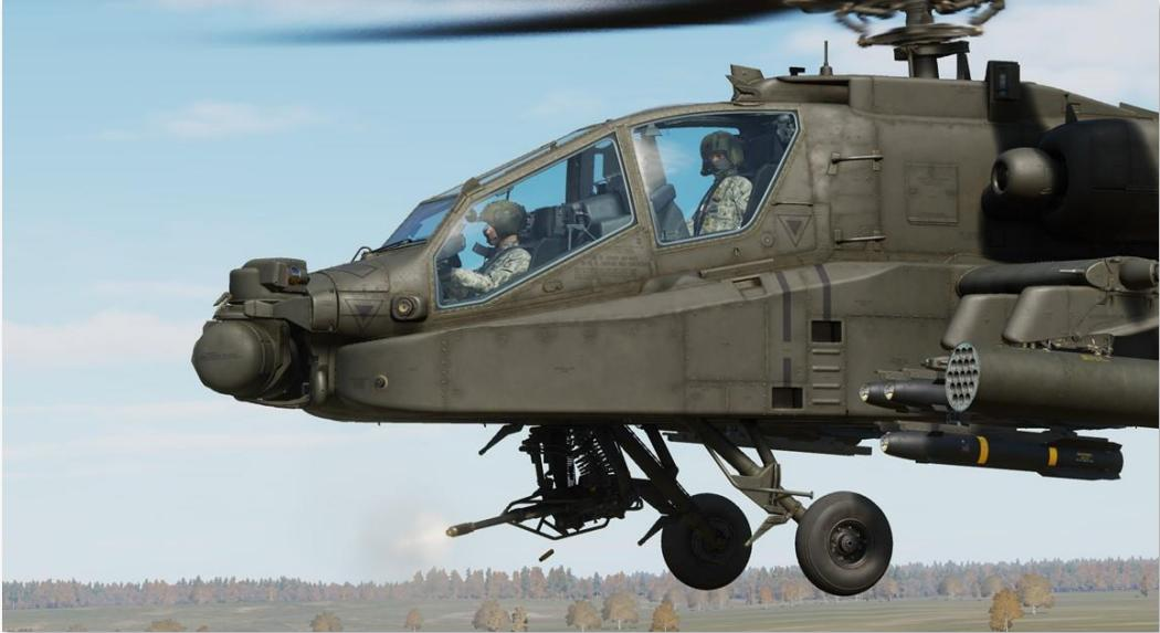
Unlike many helmet cueing systems that were post-production modifications to fixed-wing combat aircraft, the AH-64's helmet sight was designed from the beginning to function as both the primary display for flight information and as an independent but integrated targeting system.
