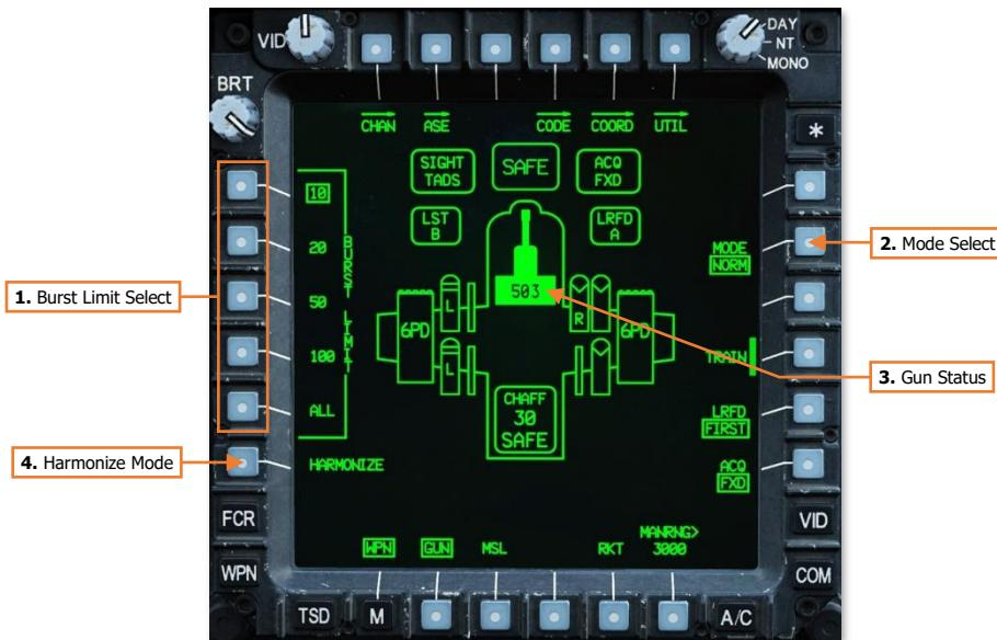
1. **Burst Limit Select.** Displays the quantity of 30mm rounds that will be fired each time the weapon trigger is pulled and held. When the burst limit is reached, a subsequent trigger pull is required to fire a subsequent burst. This setting is independent between crewstations.
