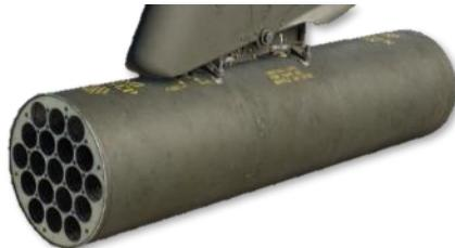
The Hydra-70 rocket family is typically employed with the Mk 66 motor, with many different warhead options available. Variants employed by the U.S. Army include the following:
