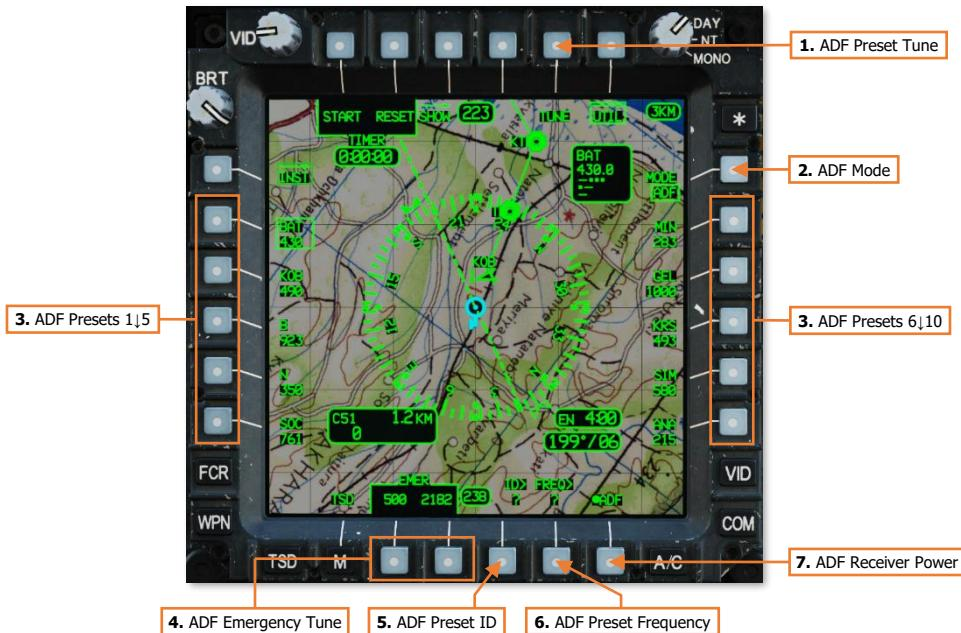
1. **ADF Preset Tune.** Tunes the ADF receiver to the selected ADF Preset.
