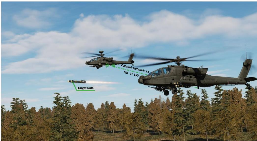
RFHO datalink messages may be sent to any AH-64D Primary member(s) within the selected datalink network, allowing the receiving aircraft to engage the FCR target with RF missiles, rockets, or 30mm gunfire, regardless of whether the receiving aircraft is equipped with an FCR themselves. However, if received by an AH-64D that is equipped with an FCR, the RFHO data will replace any target data generated by the receiving aircraft's own FCR.
