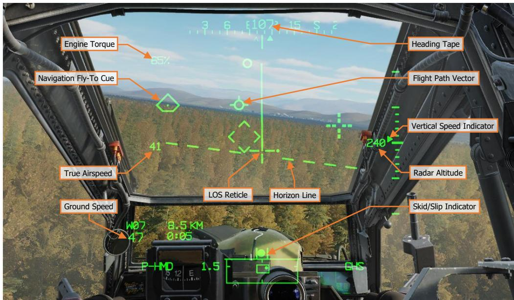
The Heading Tape along the top of the helmet display symbology can be used to monitor heading. The chevron along the bottom of the Heading Tape shows the relative direction to your next waypoint. If you turn the aircraft toward it and then align the Flight Path Vector with the Navigation Fly-To Cue, you will be flying to your waypoint.
