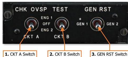
2. **CKT B Switch.** Tests the overspeed protection Circuit B for each engine.
