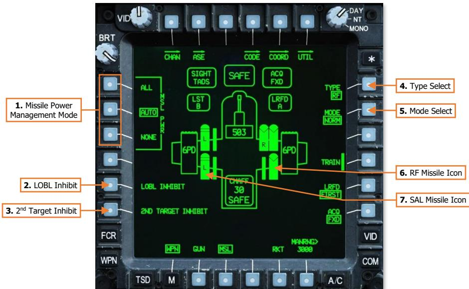
1. **Missile Power Management Mode.** When the Mode is set to NORM, selects the power management setting for all AGM-114L missiles loaded on the aircraft. This setting is common between crewstations.
