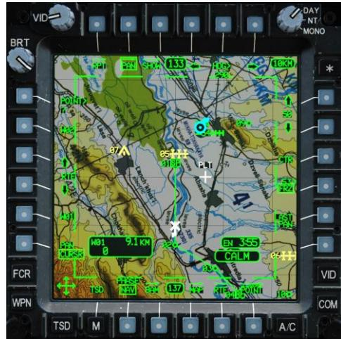
**Panning to each subsequent Route Point (Left) and continuously in reverse (Right)**
