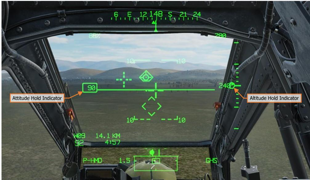
When Altitude Hold is enabled, a "home plate" box will be placed around the VSI indicator in the HDU Flight symbology and on the FLT page; and either the "RAD ALT HOLD" or the "BAR ALT HOLD" advisory will be displayed on the EUFD, depending on what Altitude Hold sub-mode is entered.
