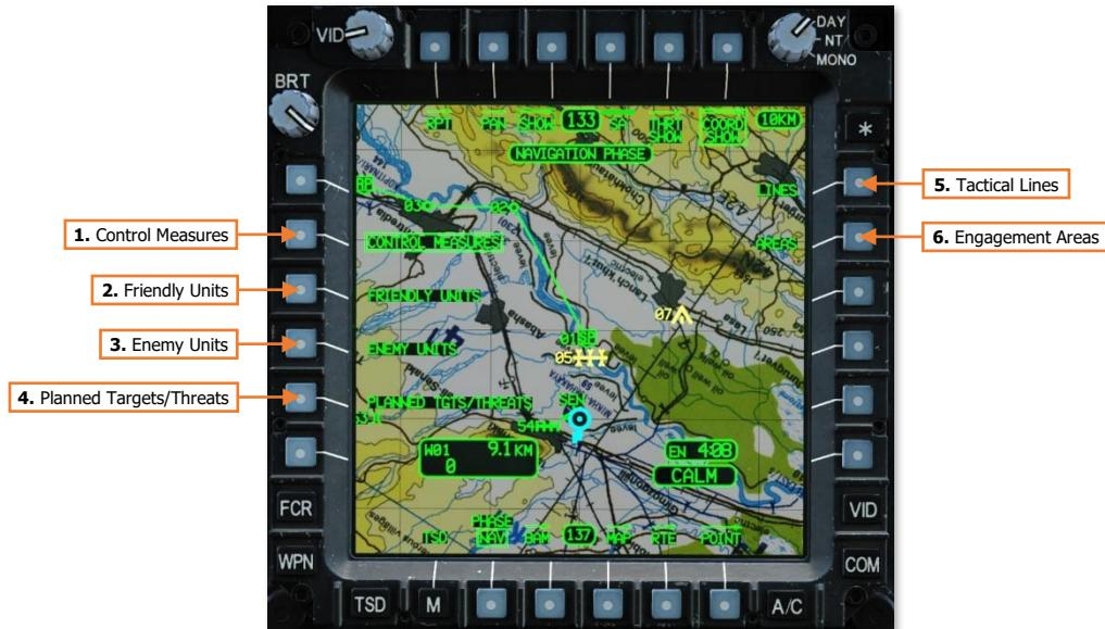
1. **Control Measures.** Enables/disables the display of general control measures. General control measures that are part of the current route, the navigation destination, or set as the acquisition source will be shown on the TSD regardless of this option.
