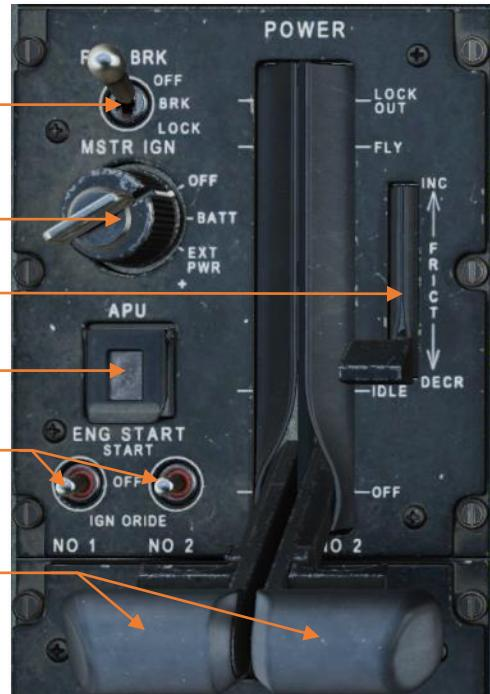
Rotor brake operation is electronically inhibited if either ENG POWER lever is beyond the IDLE position.
