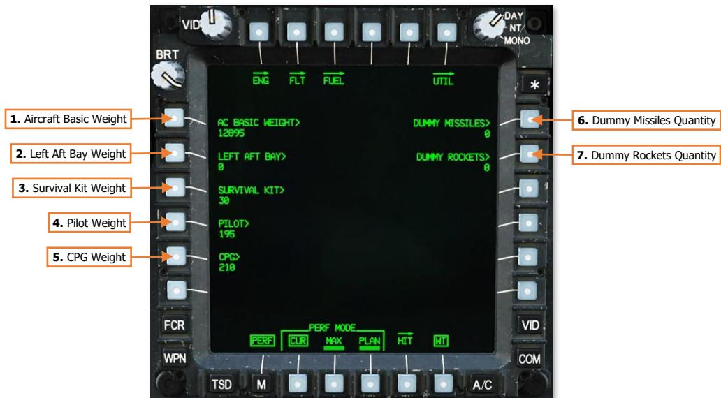
1. **Aircraft Basic Weight.** Activates the KU for inputting the basic weight and moment of the aircraft. The basic weight includes the weight of the aircraft itself, permanently installed equipment, hydraulic fluid, engine and transmission oil, and unusable fuel.
