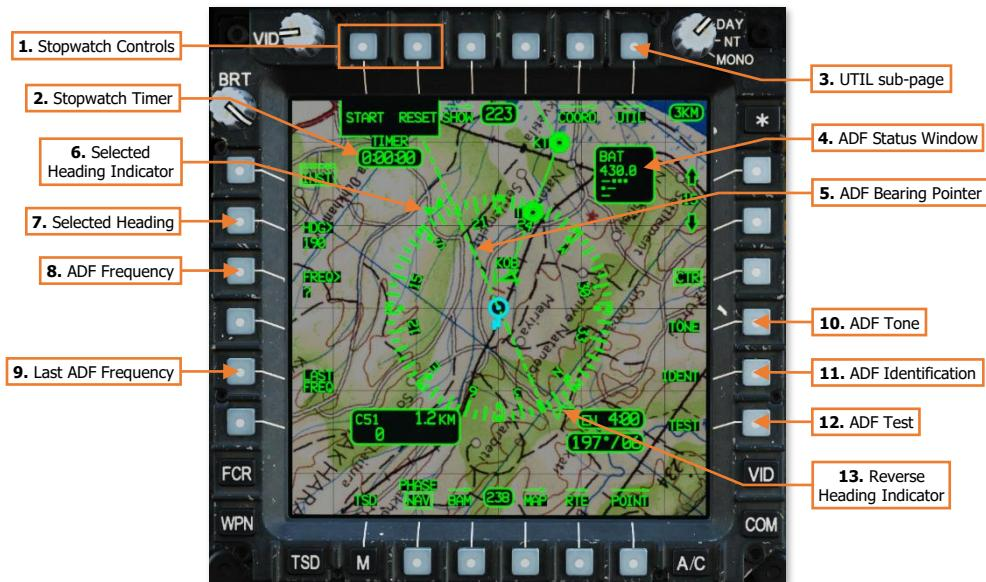
1. **Stopwatch Controls.** Controls the stopwatch timer within the crewstation.
