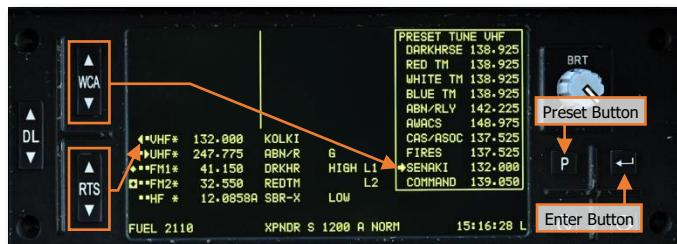
The EUFD Preset function can be useful to tune a radio without changing an MPD to the COM page. The Preset function on EUFD is limited to tuning single-channel frequencies only and cannot be used to tune frequency-hopping nets.
