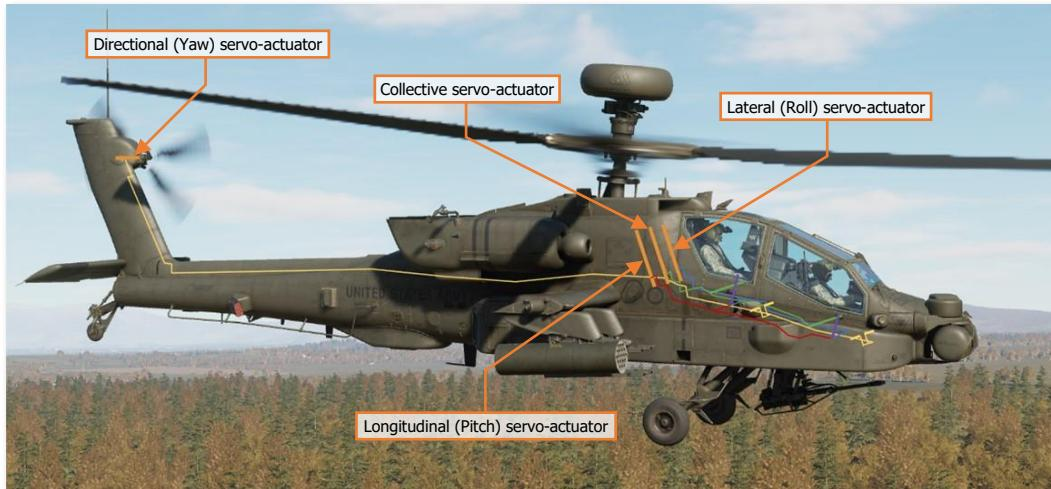
Hydraulic augmentation is provided by the Stability and Command Augmentation System (SCAS), which consists of electro-hydraulic actuators commanded by the Flight Management Computer (FMC). The FMC provides rate damping and enhanced aircraft stability for accurate weapons employment; and command augmentation for immediate, smooth, and consistent control feel across the full range of helicopter airspeeds. The FMC also provides attitude and altitude hold capability for limited hands-off flying.
