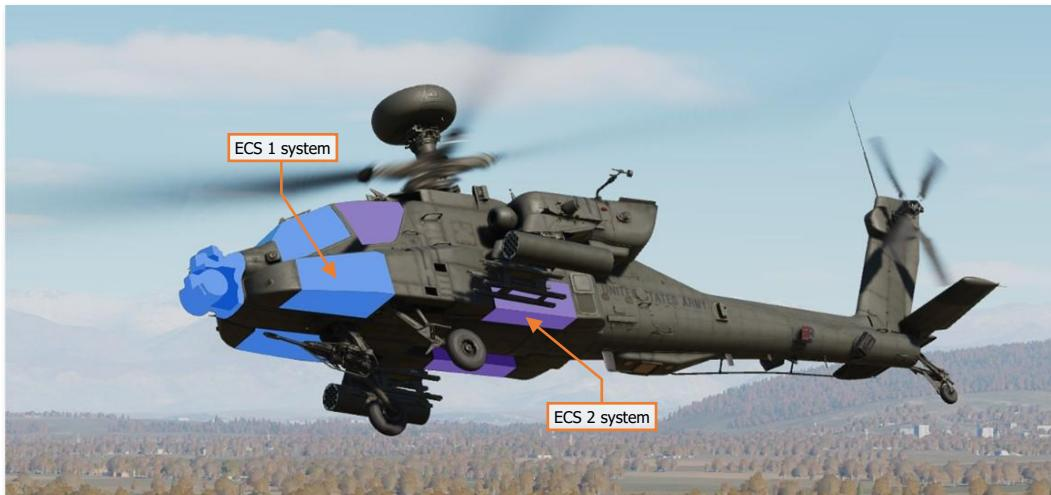
In the event of a failure of one of the ECS systems, the DCU of the functioning system will automatically open an interconnect valve between the two cockpits. The ventilation fans in the failed cockpit will stop, and the functional cockpit's ventilation fans will force cooled air into both cockpits.
