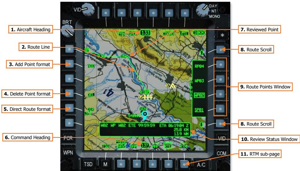
1. **Aircraft Heading.** Displays a digital readout of the aircraft's current magnetic heading in 1° increments.
