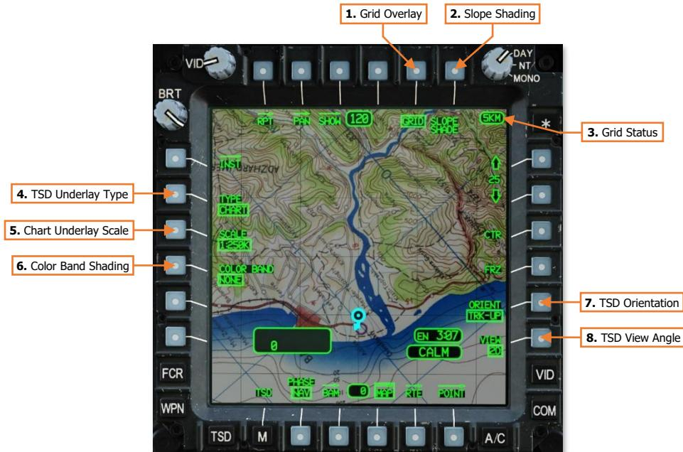
1. **Grid Overlay.** Enables/disables the grid overlay on the TSD.
