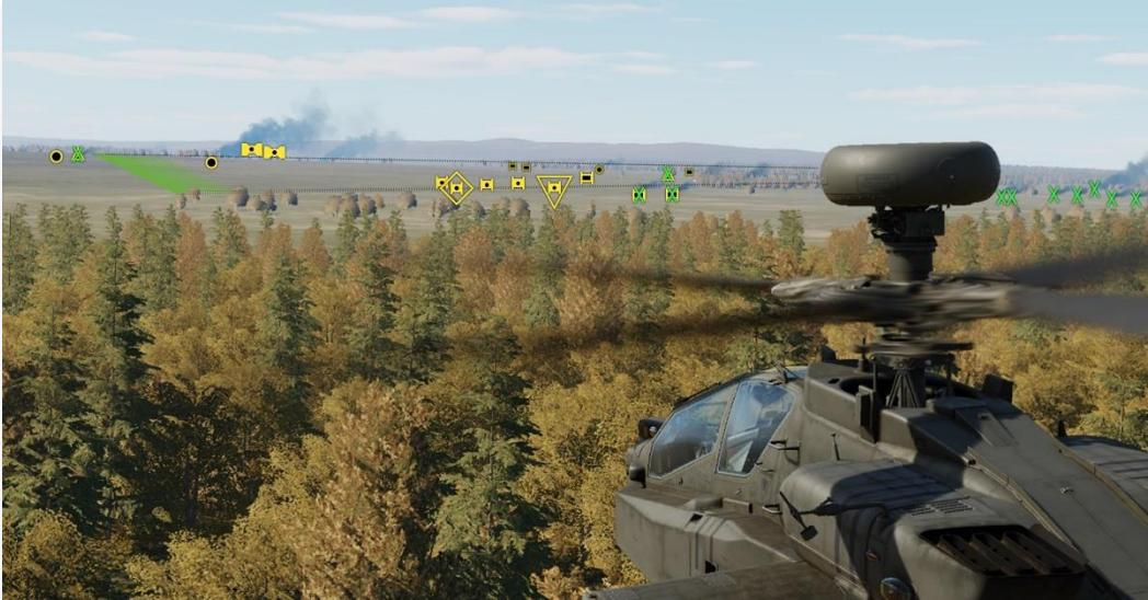
As the FCR is a sight like the HMD and the TADS, the FCR may be used to employ all three weapon systems of the AH-64D. However, it is not capable of providing guidance to the AGM-114K laser-guided missiles and can only provide target data to the AGM-114L radar-guided missile variants.
